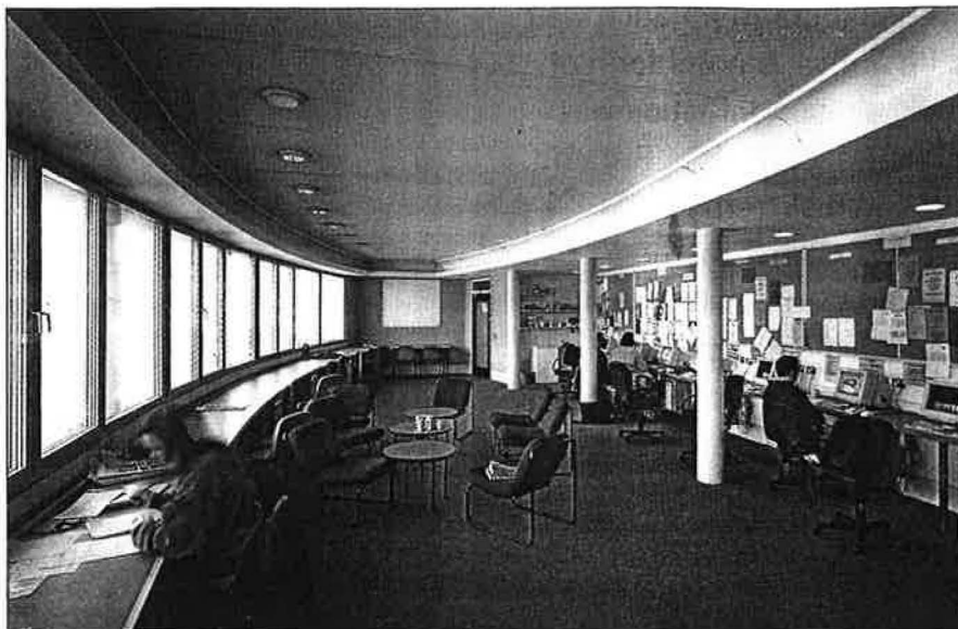
An IT resource room is located directly above the main entrance, and follows the gentle curve of the elevation. Note the row of annular soffit diffusers connecting directly to the exposed Termodeck slabs.
