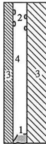
Figure 5.2: Moisture Storage in Cavities of Screened Walls
