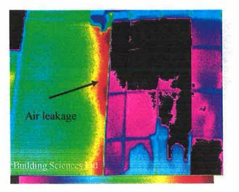
This colour image shows severe air leakage between two construction systems on a new build project. Individually the glazed curtain walling (green) and stone cladding (purple) appear to be performing well but the junction between the two has failed. The large red flare indicates the extent and of air leakage along the joint.
