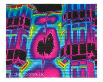
Severe air leakage at the cladding joints led to condensation and corrosion. This is identified by the red and green patterns. The mechanical systems within this building could not be properly balanced due to the loss of air occurring through the external wall at the plenum floors.
