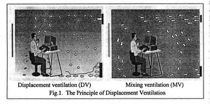
system are well documented.<sup>[1][2][3]</sup> A displacement system can achieve a high ventilation effectiveness when the internal sources produce both heat and contaminants, as is the case with people and some office equipment. The benefits available if these principles can be delivered in practice, are improved indoor air quality and also lower energy consumption due to lower flow rates and more free cooling, with supply temperature typically 19-21°C. The
