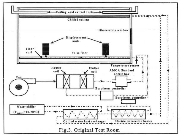
With a heat load of  $50W/m^2$  provided by PCs, 100W heaters simulating people, and a photocopier, arranged as shown in Fig. 4, and an air change rate of 9.3 per hour, the maximum output of the fan, conditions were monitored in the test room. These were compared with earlier results from the same room using standard semi-cylindrical metal diffusers when the heat load was 40 W/m<sup>2</sup> and the air change rate 3.5 per hour.
