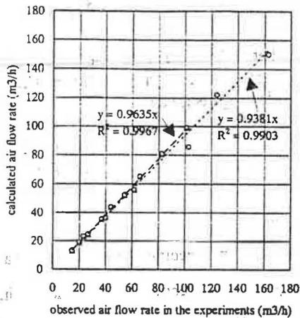
(a) Comparison between Air Flow Rates Calculated and Observed in the Experiments
