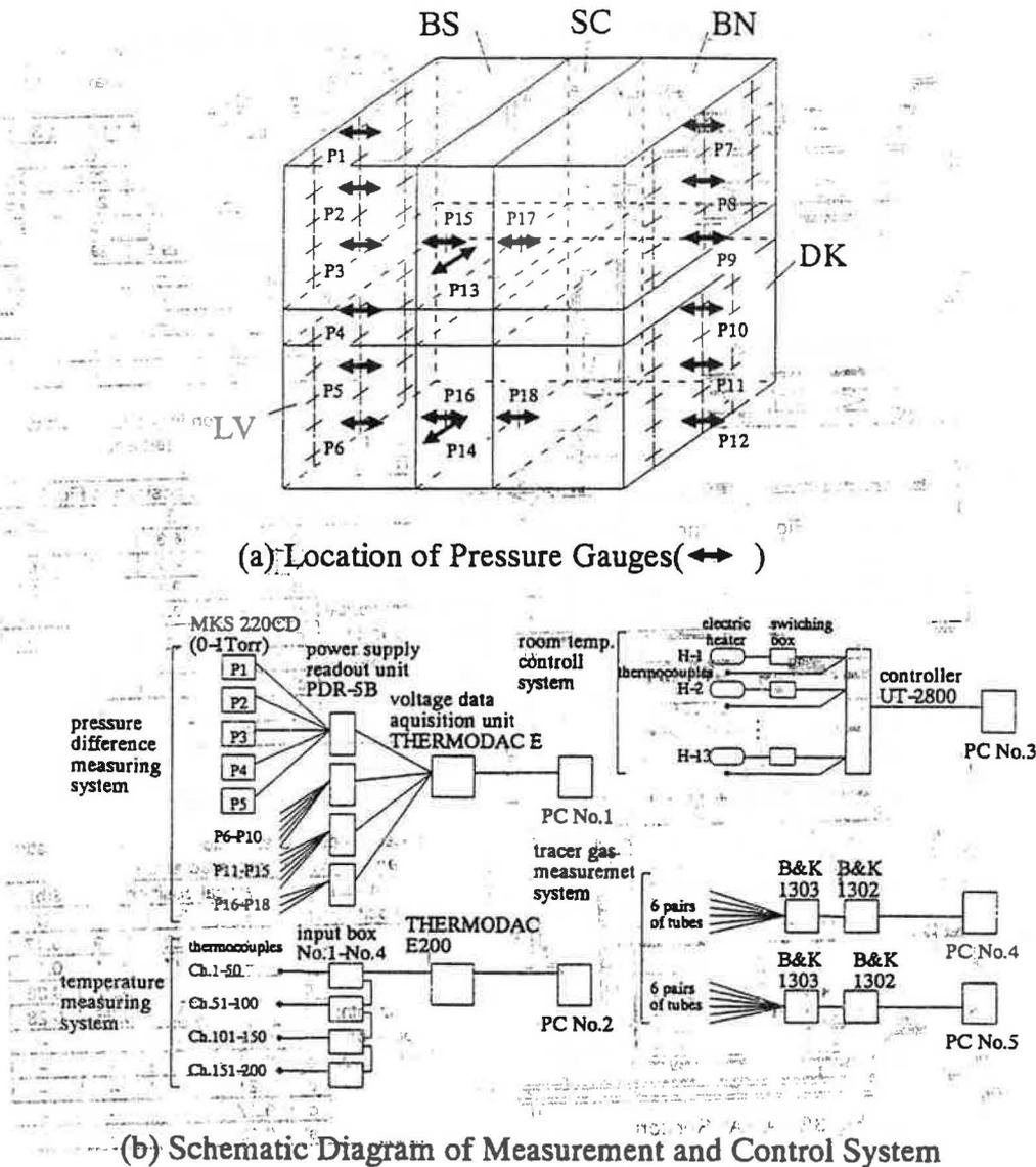
Figure 4 Measurement and control system.
