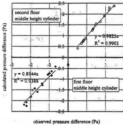
(c) Comparison of Pressure Difference at the middle height between Calculation and Observation in the Experiments
