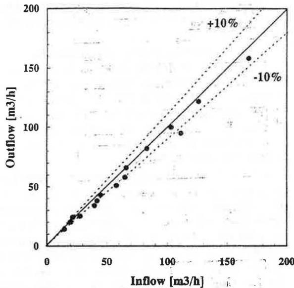
Figure 11 Comparison between inflow and outflow caused by temperature difference.
