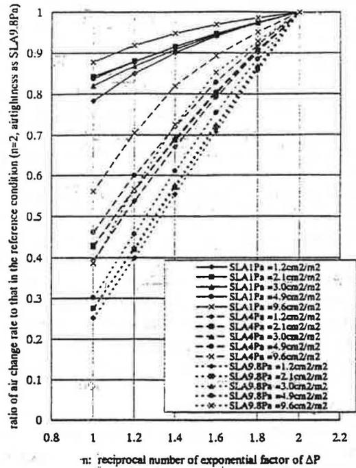
(b) dependence of air change rate on the reciprocal number of exponential factor of  $\Delta P$ , reference pressure and airtightness at 10 deg.K temperature difference
