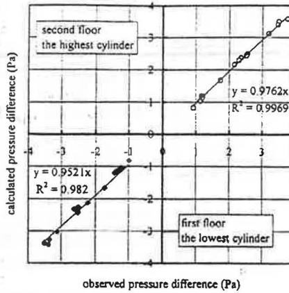
(b) Comparison of Pressure Difference between Calculation and Observation in the Experiments
