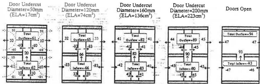
(a) Air Flow Rate (m<sup>3</sup>/h) through Cylinders due to Stack Pressure, with Partitions of Different Flow Resistance, with the Envelope Airtightness of 4.9cm<sup>2</sup>/m<sup>2</sup> (SLA<sub>9.8</sub>), under 20 K Indoor-Outdoor Temperature Difference
