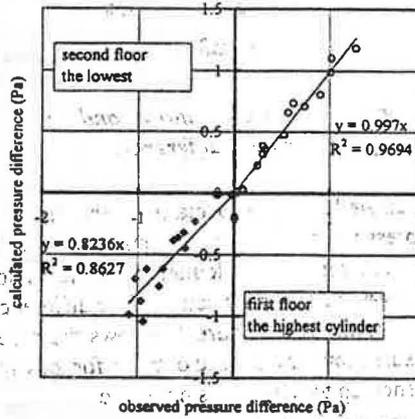
(d) Comparison of Pressure Difference between Calculation and Observation in the Experiments
