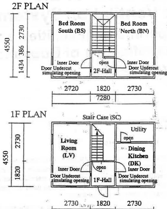
Figure 1 Plan of cylinder house.
