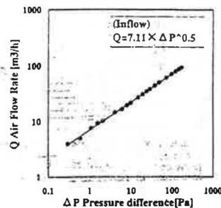
(b) Q-ΔP Characteristics of Cylinder for Inward Air Flow (at 21.0 °C, 755.7 mmHg, 65%rh)
