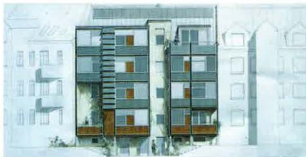
THE YELLOW HOUSE IN AALBORG (DENMARK) – DESIGN FOR GLAZED BALCONIES. RENOVATION COMPLETED IN 1997
