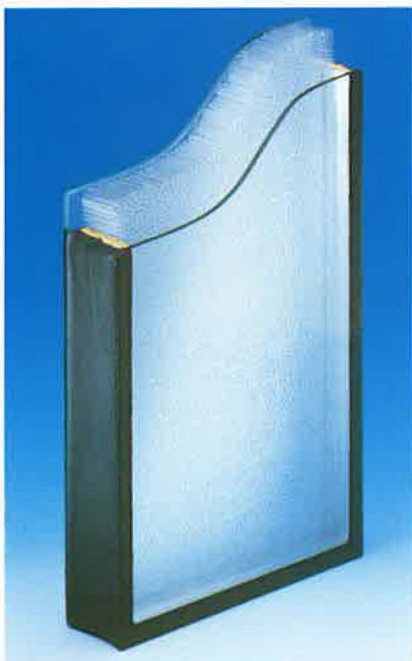
SEALED TI GLAZING: 1 OUTSIDE GLAZING 5 MM; 2 TI MATERIAL – 40 MM ACRYLIC GLASS CAPILLARY PLATE; 3 INSIDE GLAZING 4 MM WITH LOW-E COATING; 4 SPACER; 5 GASKET; 6 RARE-GAS FILL
