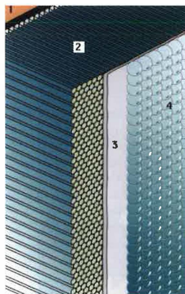
TI COMPOUND SYSTEM: 1 FIXING – GLUING WITH DARK MORTAR (ABSORBER); 2 INSULATION – CAPILLARY PLATES (POLYCARBONATE); 3 REINFORCEMENT – GLASS FABRIC AND TRANSPARENT GLUE; 4 PROTECTIVE COVER – GLASS PLASTER
