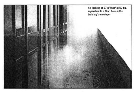
Building components such as doors and windows have long been subjected to laboratory-based rain and wind pressure testing. Whole building air leakage is a much newer concept, but the trend is clearly towards fan pressurisation of the building and measuring the airflow at a given pressure drop between the inside and outside of the building.
