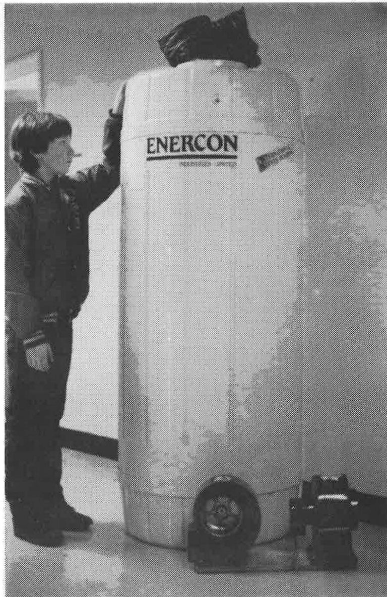
FIG. 13 A Canadian manufactured residential heat exchanger, Enercon, [8], similar in design to the Besant unit. The supply and exhaust fans included with the unit are also shown.
