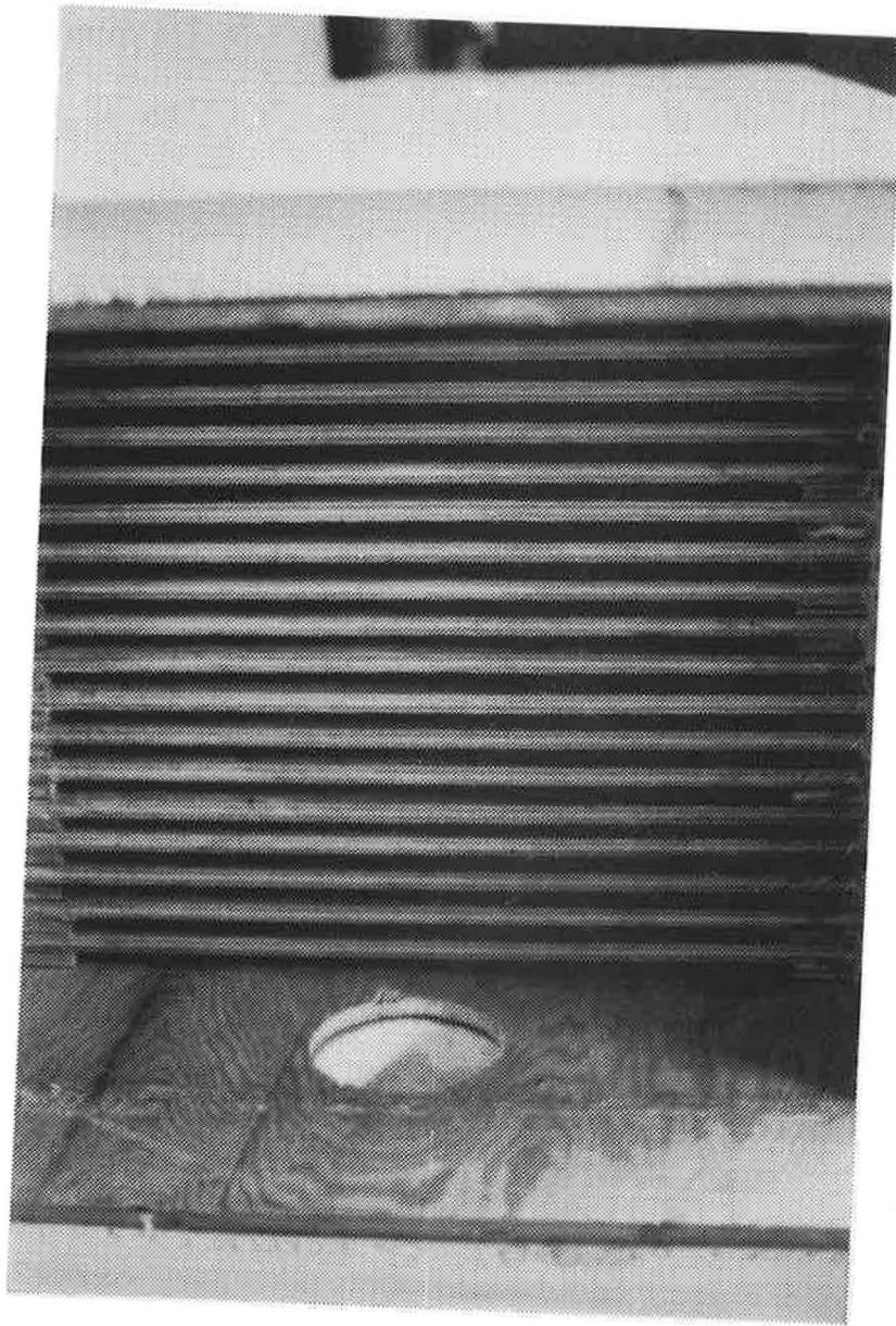
FIG. 12 Internal View of Heat Exchanger Shown in Fig. 11. The 1/2 inch plywood spacers separating the 6 mil polyethylene sheets which serve as the heat transfer surface are shown.
