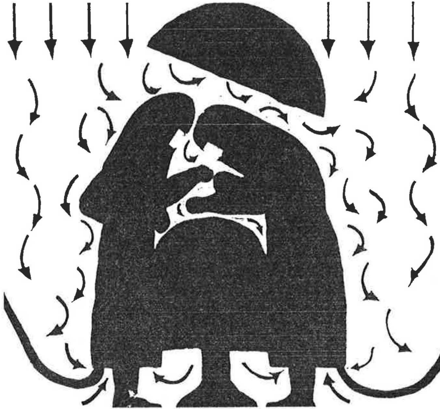
Fig. 7. Semiturbulent air flow combined with body exhaust system. Turbulence not sufficient to permit currents rising from the floor. Perfect overhead surgical lighting possible.
