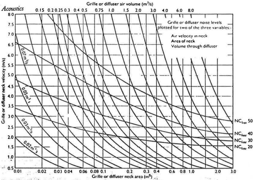
Figure 10 Guidance on flow-generated noise for diffuser/grille
