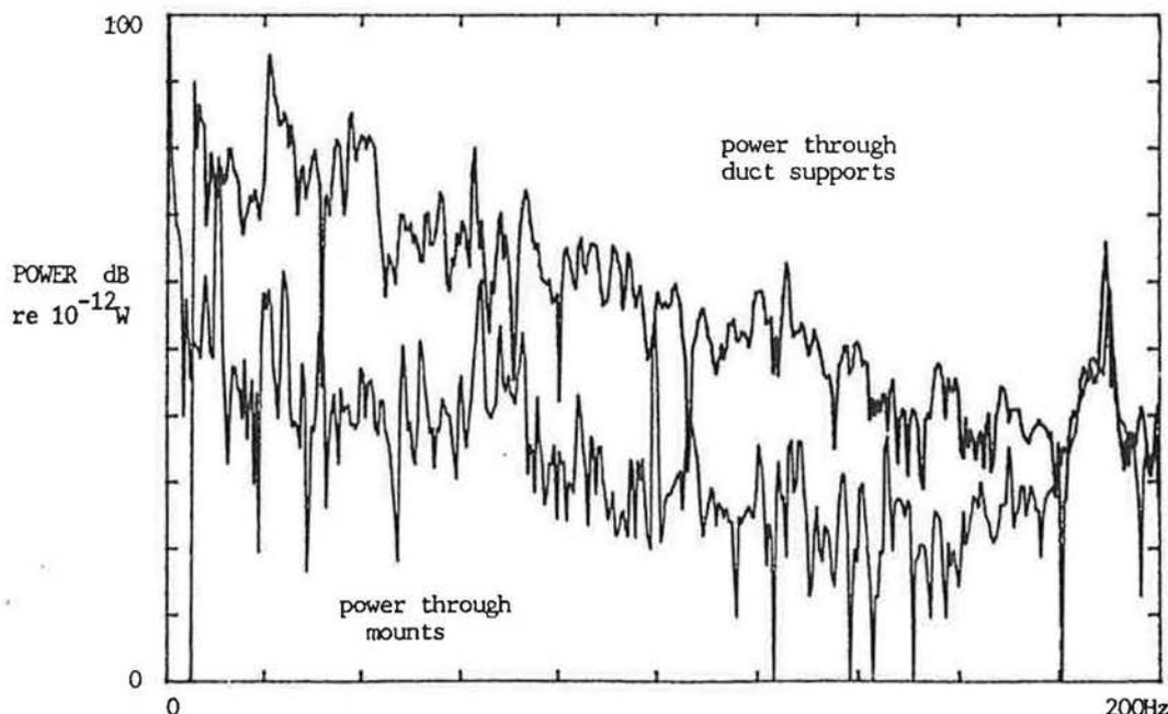
Figure 19 Comparison of power flow through mounts and through duct supports
