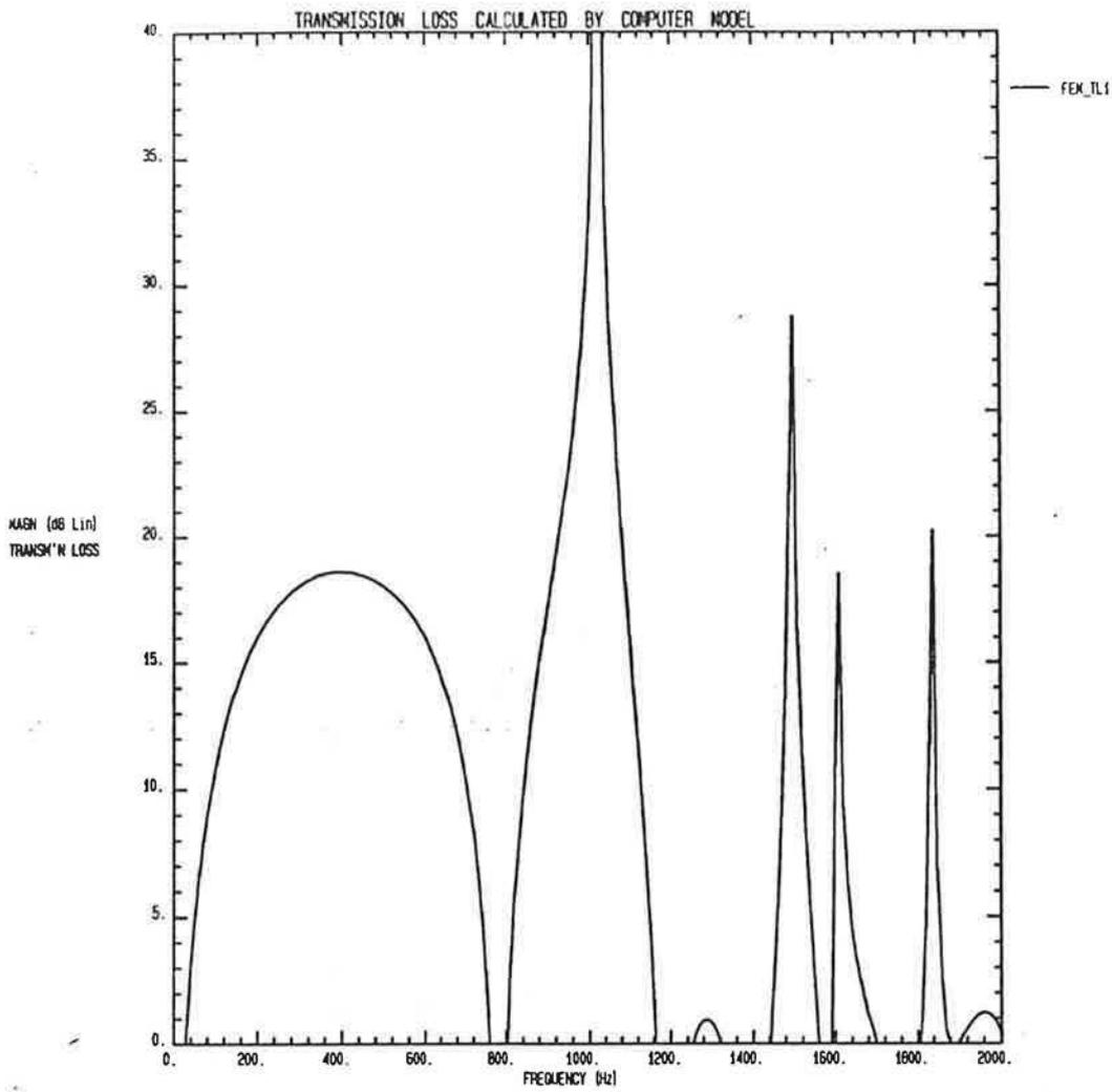
Figure 23 Results for plenum of Figure 21 from SYSNOISE program<sup>(9)</sup>
