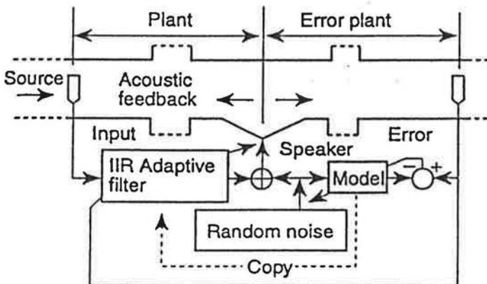
Figure 31 Active noise control schematic and block diagram
