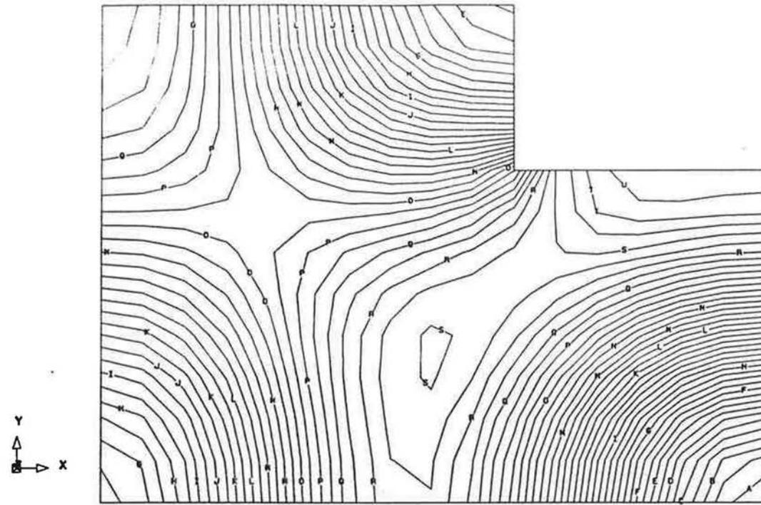
Figure 27 Acoustic finite-element analysis: Mode in a small room (101 Hz)
