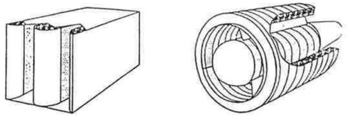
Figure 32 Conventional passive silencers
