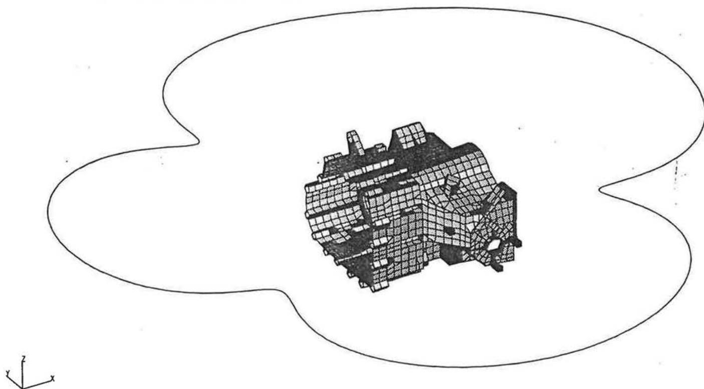
Figure 26 Directivity diagram of sound pressures around a gearbox, superimposed on a BE mesh of the component
