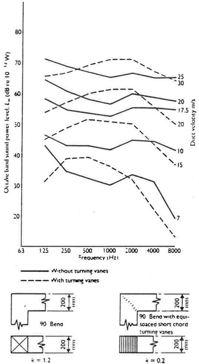
Figure 7 Sound power spectra produced by 90° elbows in a 200 mm × 200 mm duct system with and without short-chord turning vanes
