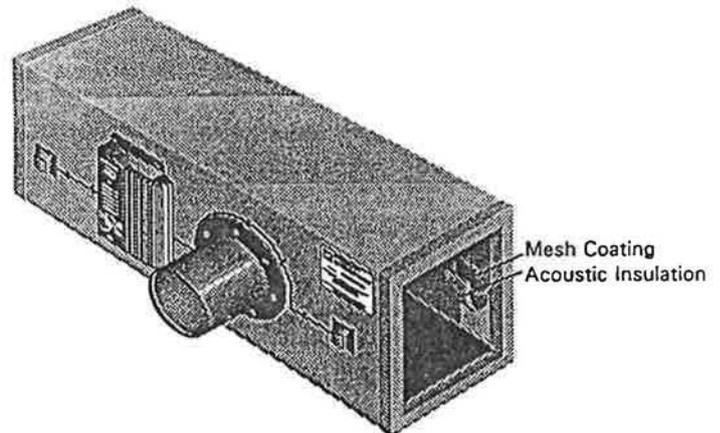
Figure 33 Active/passive hybrid duct silencer
