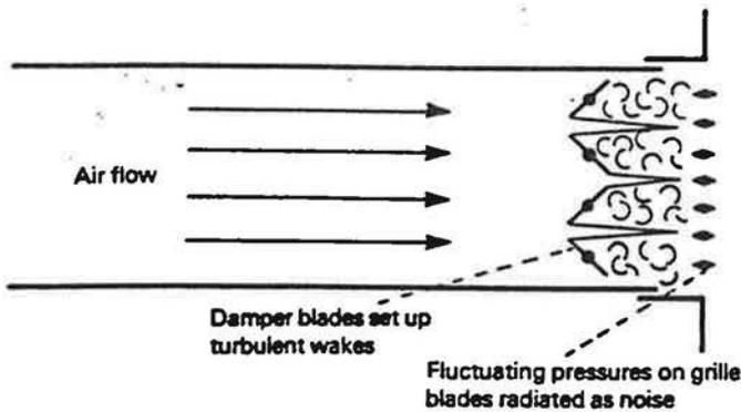
Figure 12 Mechanism of noise generation by dampers and grilles
