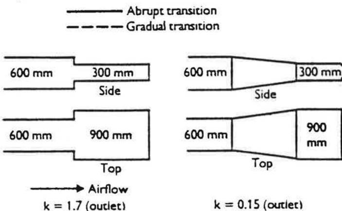
Figure 6 Sound power levels and gradual area transitions from 600 mm × 600 mm to 900 × 300 mm duct cross-section
