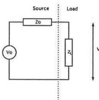
Figure 17 Voltage analogue for noise sources:
