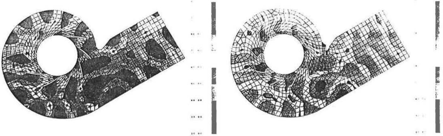
Figure 20 Sound pressure levels at 167 Hz inside a centrifugal fan
