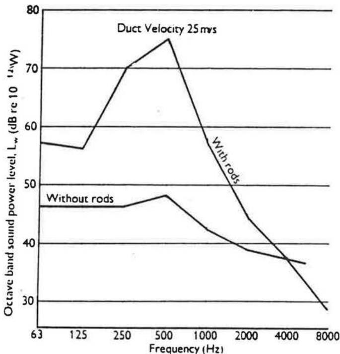
Figure 2 Sound power spectra of noise for  $600 \times 600 \text{ mm}$  duct with and without 4 off 13 mm diameter rods
