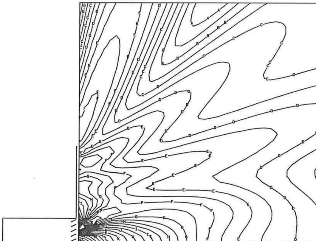
Figure 24 Sound pressure around outlet grille — 2 kHz
