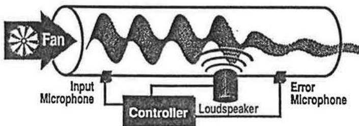
Figure 30 Active noise control in a duct
