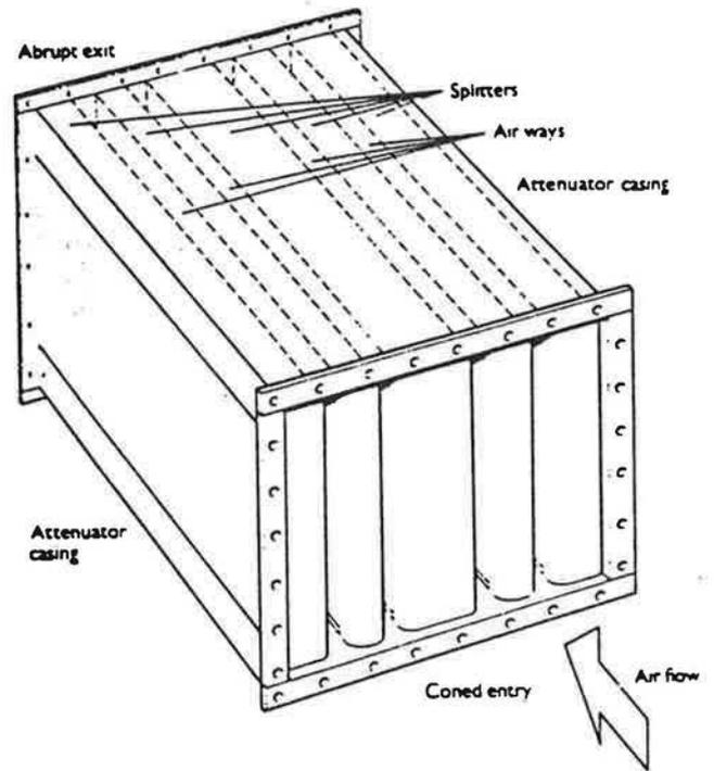
Figure 13 Rectangular attenuator
