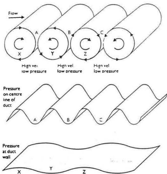
Figure 8 Duct buffeting
