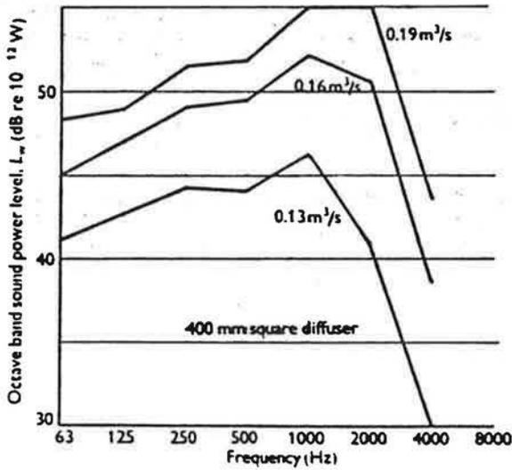
Figure 11 Diffuser sound power level
