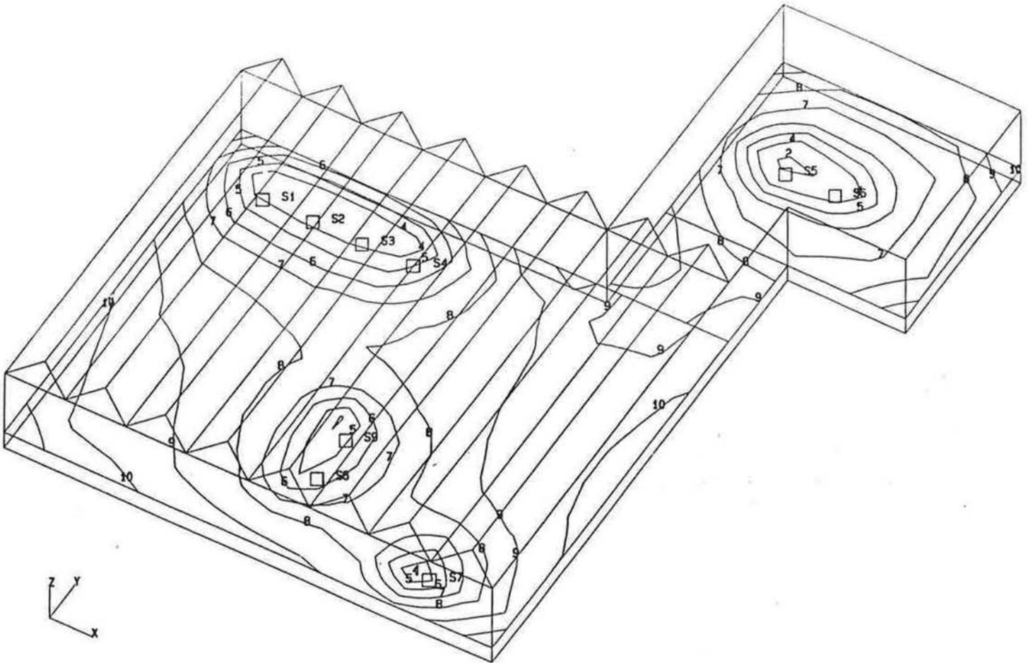
Figure 29 .Noise contours for plant room (See Table 2 for key)
