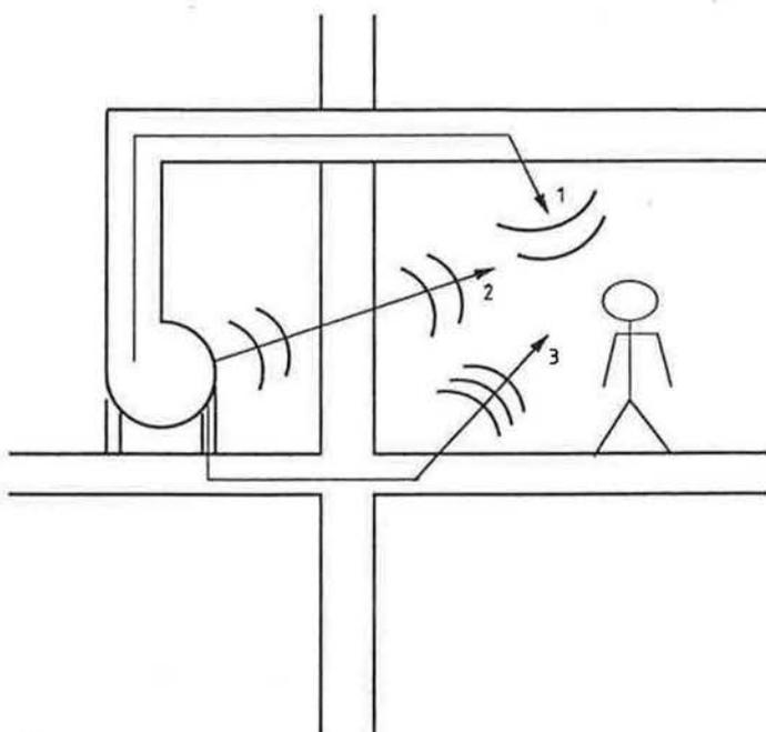
Figure 16 Sound transmission from a machine to a receiver: Path 1 duct-borne; Path 2 airborne; Path 3 structure-borne
