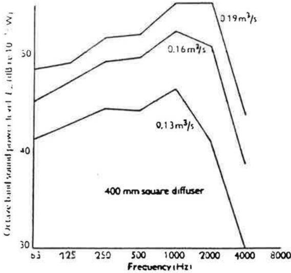
Figure 5 Diffuser sound power level
