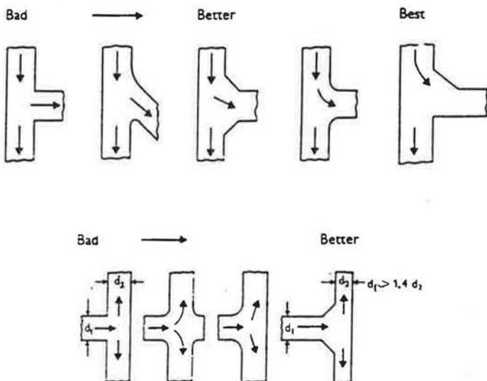
Figure 9 Guidelines for minimising flow-generated noise at branchings and take-offs
