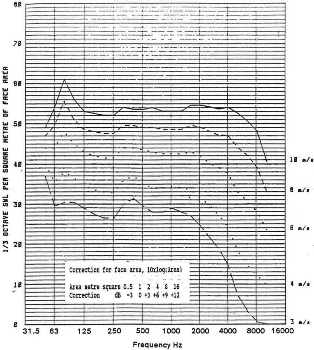
Figure 15 Rectangular attenuator outlet flow noise
