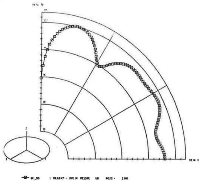
Figure 25 Directional effects of outlet grille construction — 2kHz
