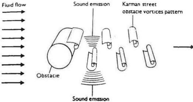
Figure 1 Formation of turbulence
