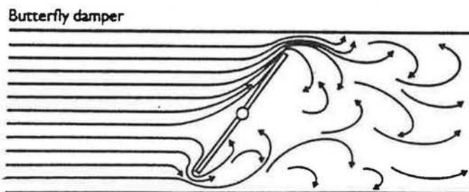
Figure 4 Turbulent flow behind butterfly dampers
