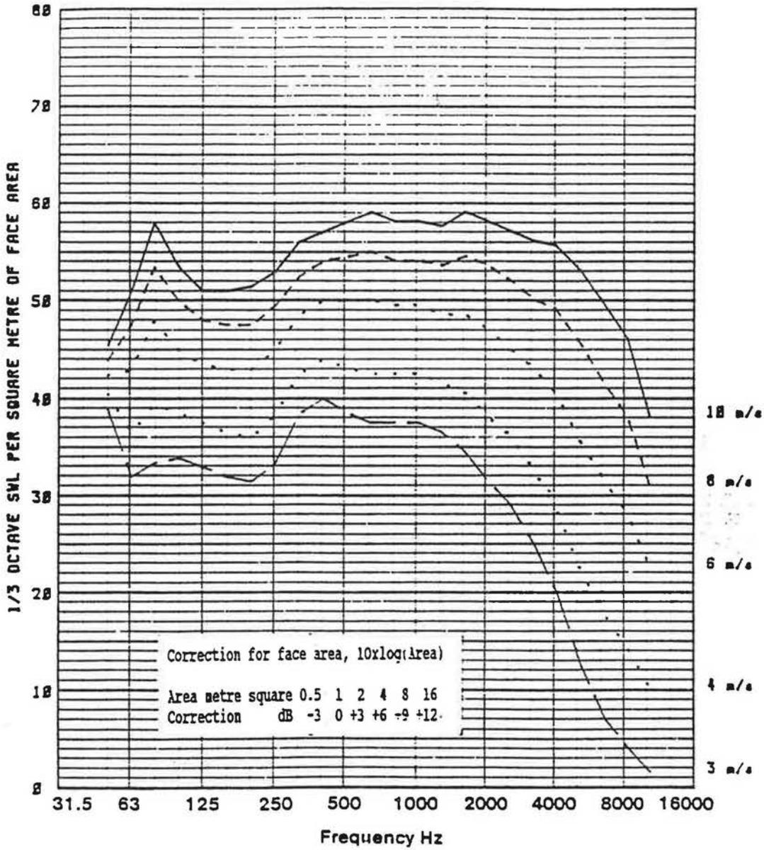
Figure 14 Rectangular attenuator inlet flow noise
