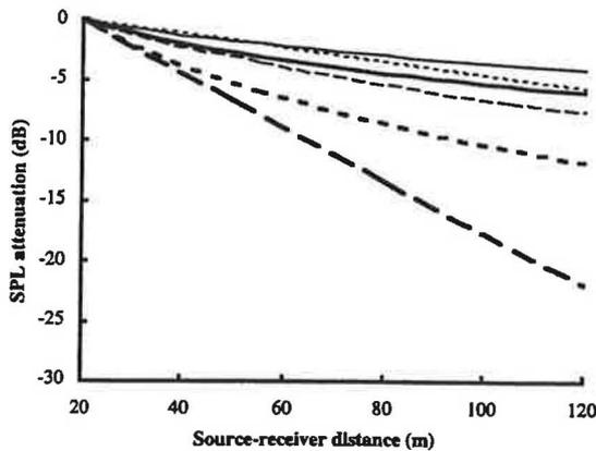
Fig. 1. SPL attenuation from 20 m calculated using equation (1) (dotted:  $\alpha = 0.05$ ; thick dotted:  $\alpha = 0.2$ ), equation (8) (line:  $\alpha = 0.05$ ; thick line:  $\alpha = 0.2$ ) and equation (22) (dashed:  $\alpha = 0.05$ ; thick dashed:  $\alpha = 0.2$ ).  $S = 5$  m by 5 m.
