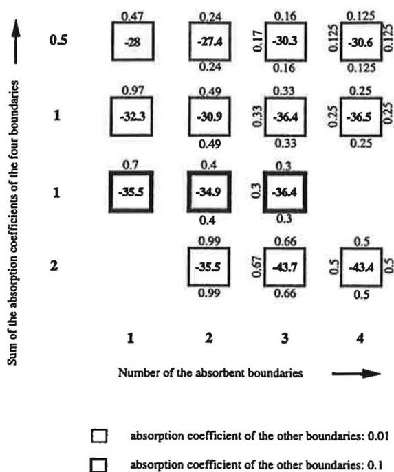
Fig. 6. SPL attenuation with reference to PWL at 120m with different absorber arrangements.  $S = 5$  m by 5 m. Calculated using equation (4).
