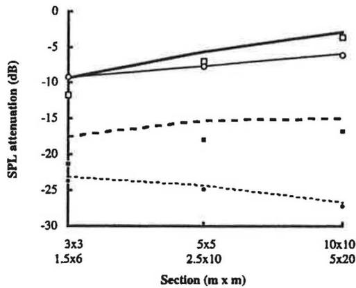
Fig. 3. SPL attenuation at 120 m from 20 m [thick line: equation (22),  $a = b$ ; square: equation (22),  $a = 4b$ ; line: equation (1),  $a = b$ ; circle: equation (1),  $a = 4b$ ] and with reference to PWL [thick dotted: equation (21),  $a = b$ ; filled square: equation (21),  $a = 4b$ ; dotted: equation (1),  $a = b$ ; point: equation (1),  $a = 4b$ ].  $\bar{\alpha} = 0.05$ .
