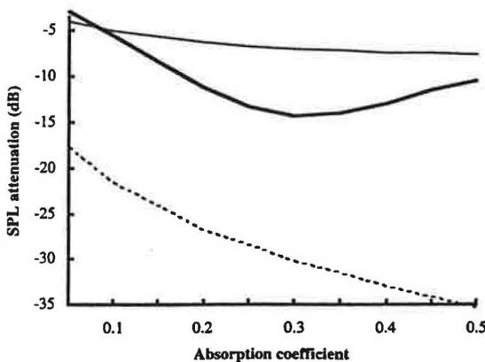
Fig. 4. SPL attenuation at 50 m with different absorption coefficients [line: equation (1), from 20 m; dotted: equation (1), with reference to PWL; thick line: equation (22), from 20 m].  $S = 3$  m by 3 m.
