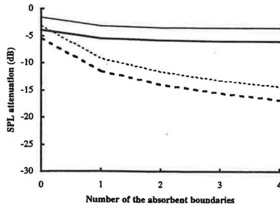
Fig. 5. SPL attenuation at 50 m (line: from 20 m; dotted: with reference to  $P_{IN}$ ) and 120 m (thick line: from 20 m; thick dotted: with reference to  $P_{IN}$ ) with different number of absorbent boundaries ( $\alpha_i = 0.8$ ).  $S = 3$  m by 3 m. Calculated using equations (9) and (11).
