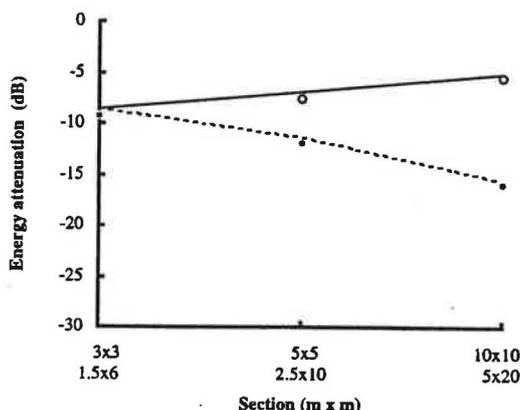
Fig. 2. Attenuation of the total energy in the whole section (line:  $a = b$ ; circle:  $a = 4b$ ) and the energy per unit area in a section (dotted:  $a = b$ ; point:  $a = 4b$ ).  $\alpha = 0.05$  and  $l_s = 120$  m. Calculated using equation (8).
