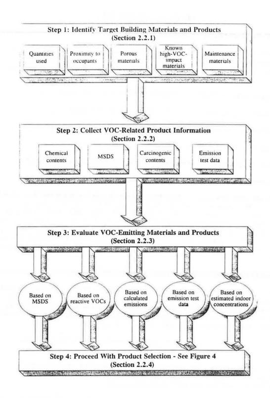
Figure 3. Four-Step Strategy for Evaluating and Selecting Building Materials and Products
