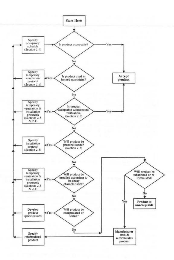
Figure 4. Flow Chart for Selecting Building Materials and Products
