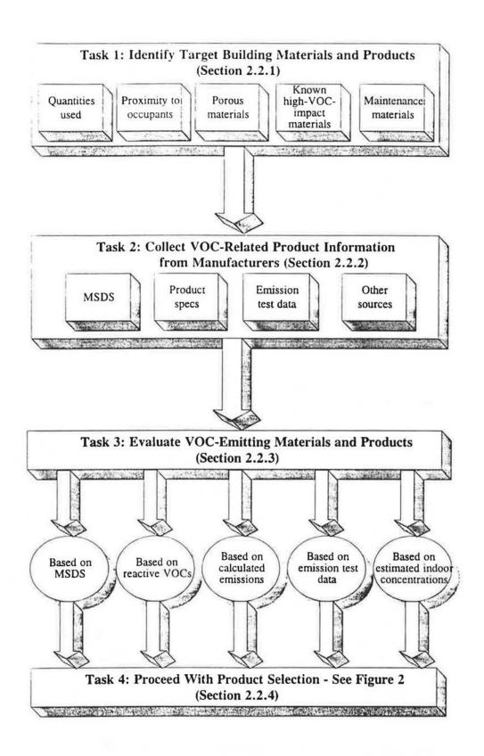
Figure 1. Four-Step Strategy for Evaluating and Selecting Building Materials and Products
