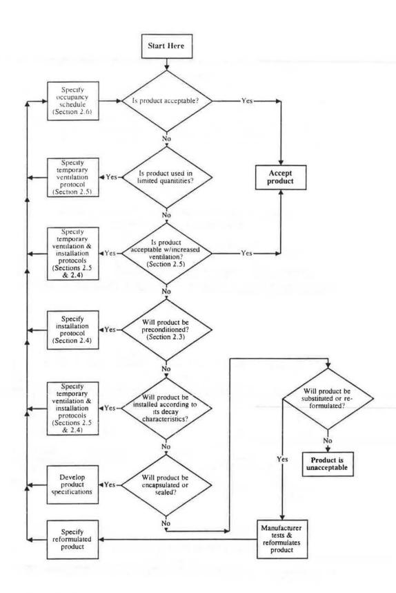
Figure 2. Flow Chart for Selecting Building Materials and Products
