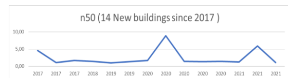
Figure 3: Results of the airtightness tests performed on 14 new buildings between 2017 and 2021
