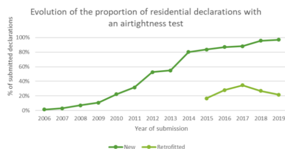
Figure 1: Evolution of the proportion of residential declarations with an airtightness test in Flanders
