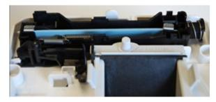
Figure 4-52 Humidity sensible exhaust unit.
