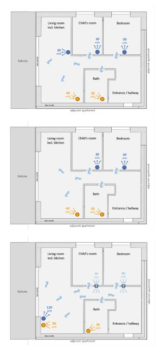
Figure 3-36 Schematic sketch of the simulated ventilation concepts. Top: Reference MVHR, Center: extended cascade ventilation, Bottom: active overflow concept.
