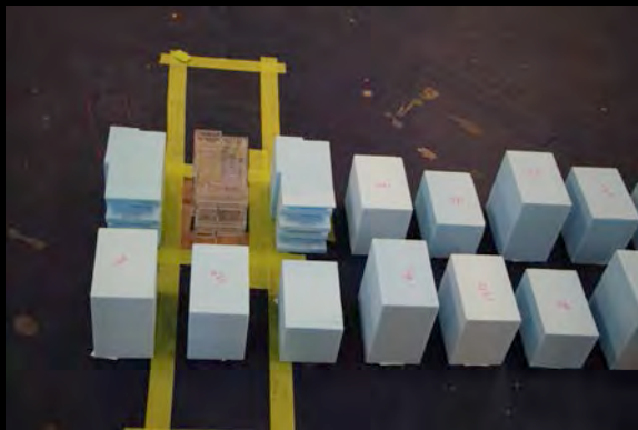
Sealed model at 1:100 scale with 299 pressure taps spread over 5 facades
