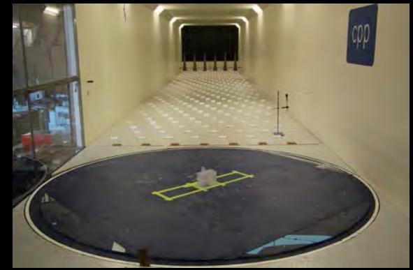
Sealed model at 1:100 scale with 299 pressure taps spread over 5 facades
