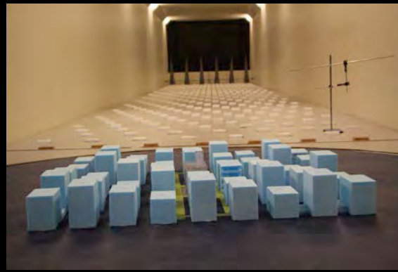
Sealed model at 1:100 scale with 299 pressure taps spread over 5 facades
