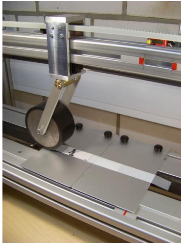
Included in draft DIN 4108 part 11: 180° peel test according to EN 1939
