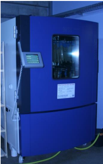
Accelerated ageing of bonding samples: Exposition to climate 65°C/80% relative humidity for 60 weeks in climate chamber at Fraunhofer IBP/University of Kassel, Germany
