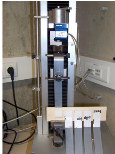
Included in draft DIN 4108 part 11: 180° peel test according to EN 1939
