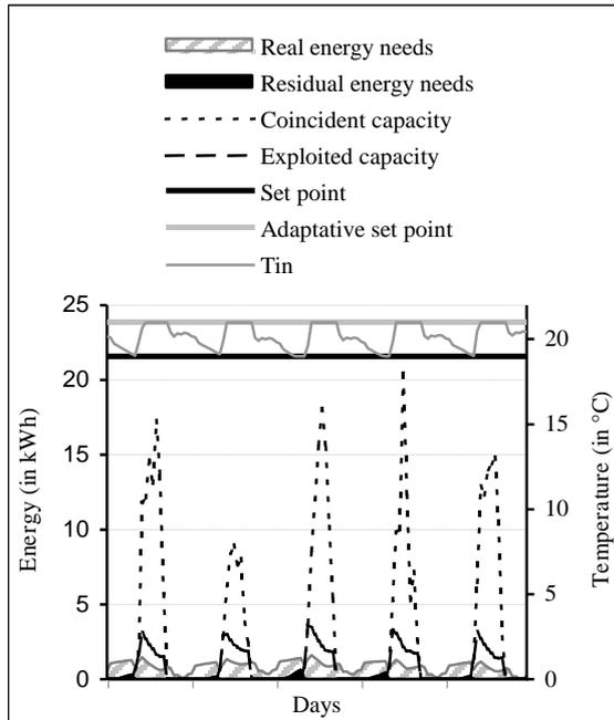
Figure 6: Principle of the adaptative set point
