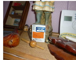
Figure 3: Room temperature and relative humidity sensor
