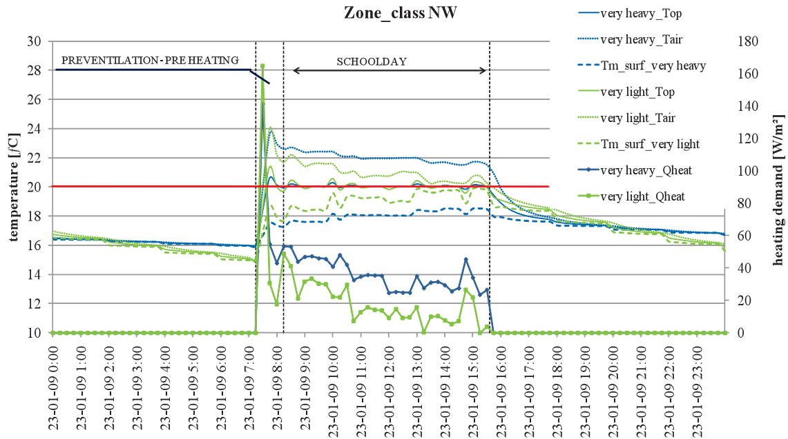
Figure 6 Heating pattern on a regular school day (Tuesday 23rd of January) in winter time for a very light and very heavy structure (calculation time step: 15 minutes)
