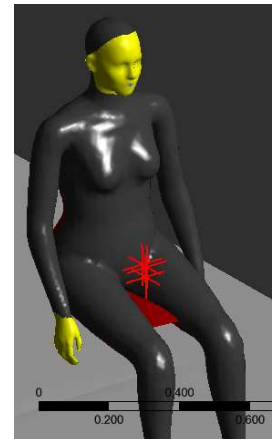
Figure 8 Points of maximum residuals located near to the chair region shown as red cross points.
