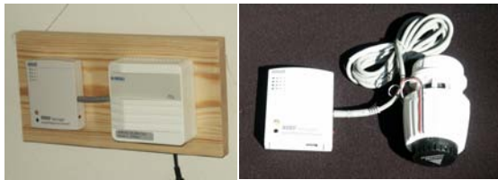
Figure 1: Pictures of the instruments used to measure the indoor environmental variables and temperature set-point of the thermostatic radiator valves.
