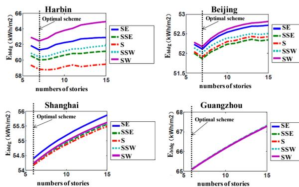
Figure 9 An example of the sensitivity analysis (upon the number of stories) based on the optimal scheme
