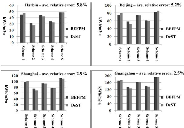
Figure 6 Accumulative cooling load prediction comparison between BEFPM and DeST
