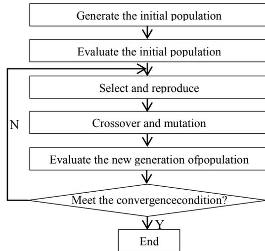
Figure 3 The standard operation flow of GA
