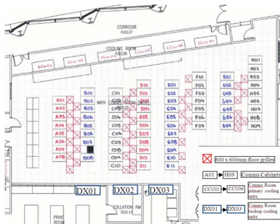
Figure 4 Primary and secondary cooling layout
