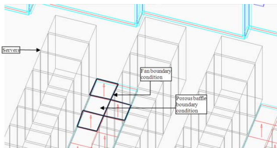
Figure 6 Fan and Porous baffle setup
