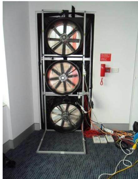
Figure 2: Blower door used for air leakage testing
