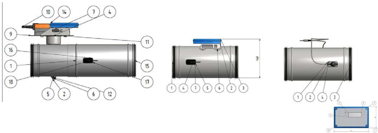
The Lindab solution is an ultrasonic measuring device with three features depending on usage. The simplest is the sensor which only contains the transmitter and receiver and has to be read by a display that is like a handheld measuring device via a USB or radio. This is mostly to be used at a commissioning and service phase.
