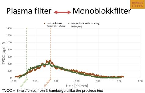
No difference between a Monoblokk filter and Plasmafilters. Our conclusion – plasma has little effect, the importance is having a good recirculation filter
