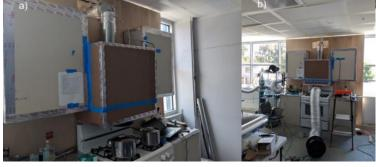
About 15% of flow missed if measurements are made for the bottom inlet only
