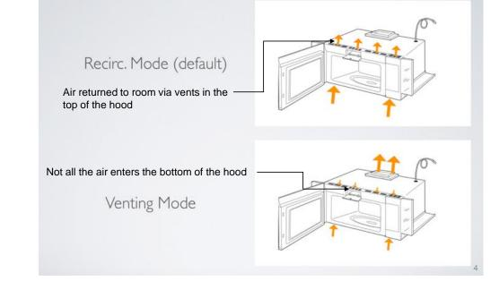
Simultaneous inlet & outlet measurements to determine correct microwave hood flows
