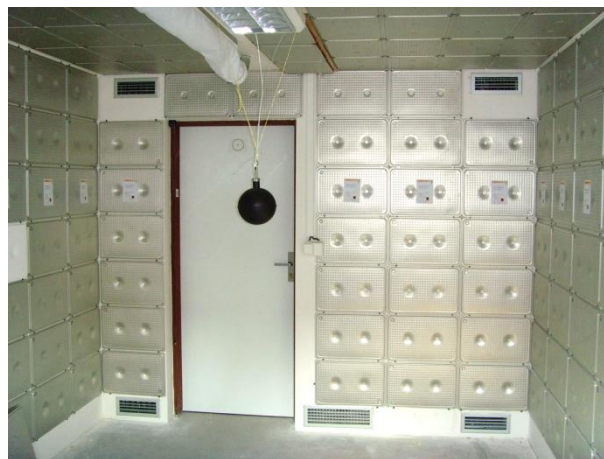
Fig. 3 Experimental room with PCM filled panels
