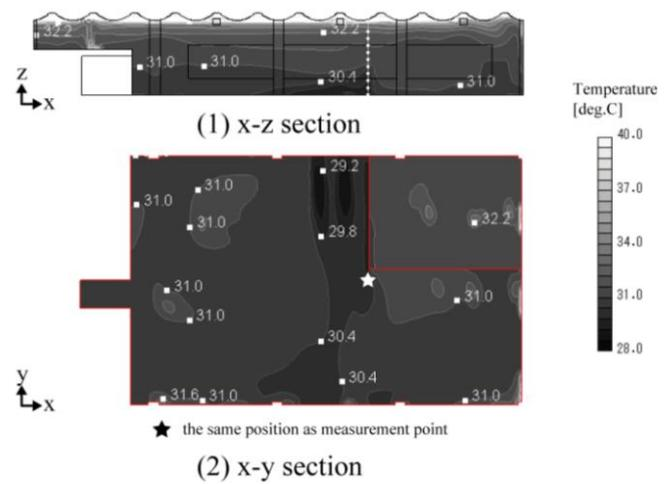
**Figure 5** Counters of temperature obtained by CFD (case 0)
