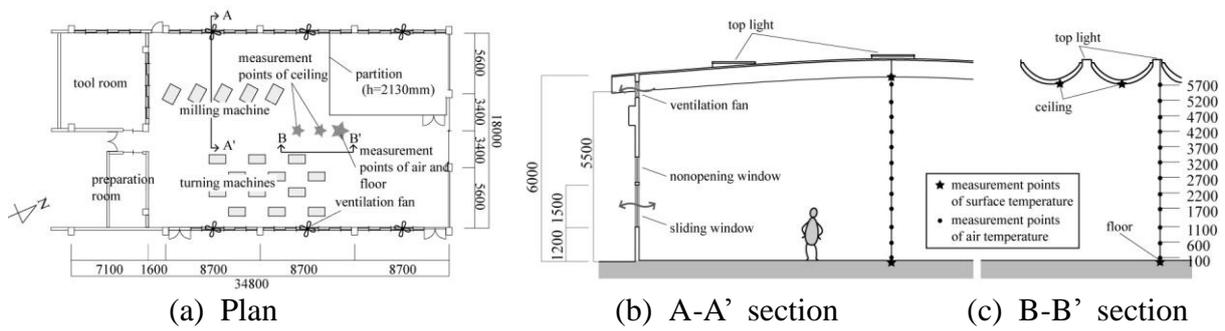
**Figure 1** Plan and Sections of the workshop and Measurement Points
