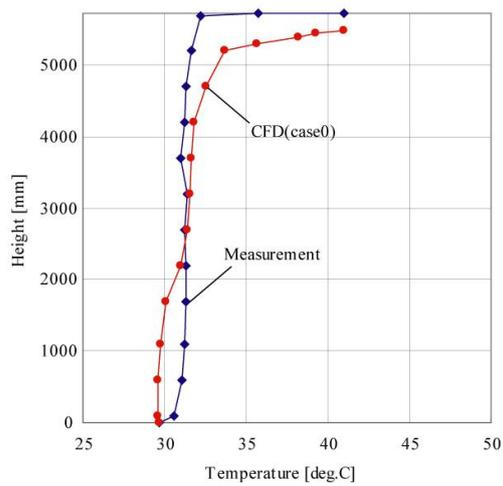
**Figure 4** Vertical temperature distributions
