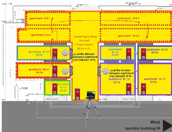
Figure 3: Sectional view of apartment building IH with 11 apartments in Iserlohn showing the test setup.
