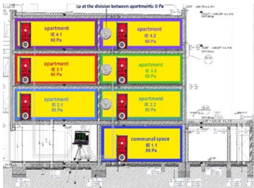
Figure 2: Sectional view of apartment building IE with six apartments and a communal space in Iserlohn showing the test setup.
