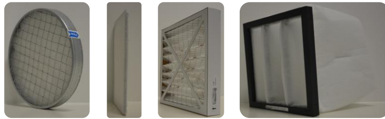
Figure 2 Pictures of the different tested filter types: A) G3 duct type, B) G4 wireframe, C) G4 folded panel, D) G4 bag type
