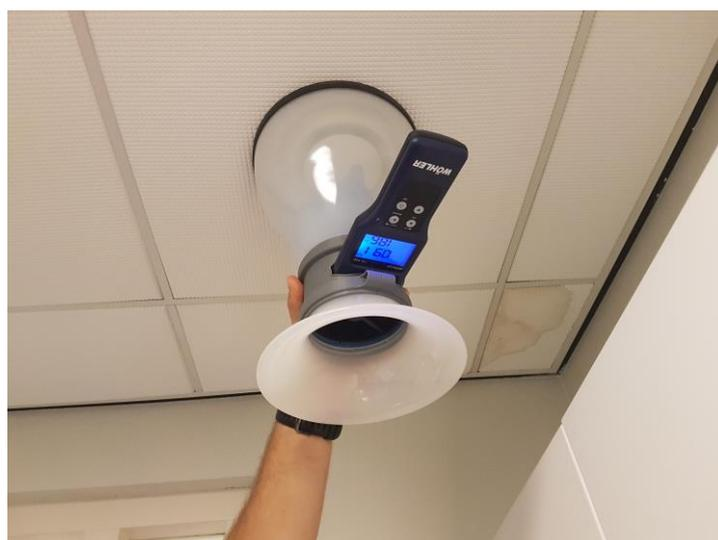
Figure 4: Passive flowmeter (prototype)
