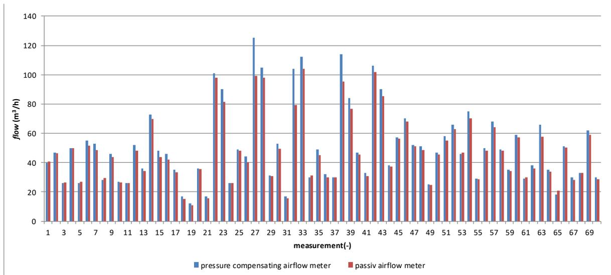
Figure 5: Comparison pressure compensating and passiv airflow meter
