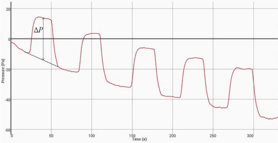
Figure 2: Typical measured pressure difference
