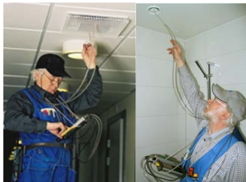
Figure 2: Example of a supply and an exhaust pressure drop air flow measurement
