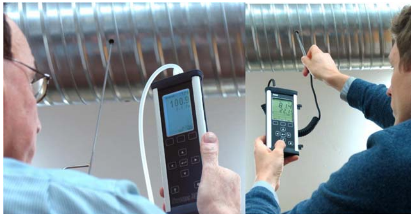
Figure 4: Pitot static tube or velocity probe points in duct method.
