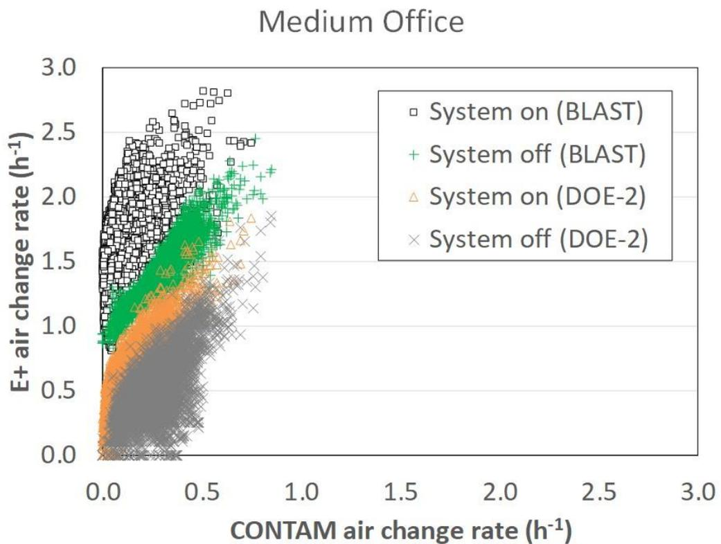
Fig. 1 EnergyPlus infiltration rates vs. CONTAM infiltration rates for Medium Office building using (a) NIST correlations and (b) DOE-2 and BLAST coefficients
