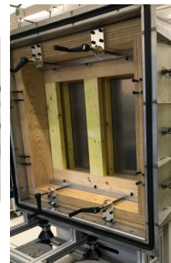
Figure 2c : the sample holder
