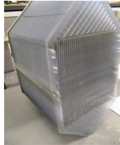
Figure 4 Condensate build-up within the exhaust ducts of the HR block
