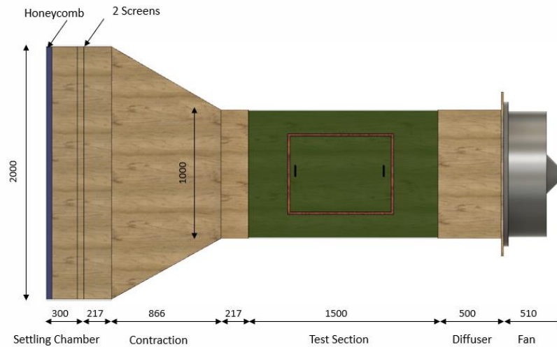
Figure 2: Final dimension of wind tunnel [in mm]
