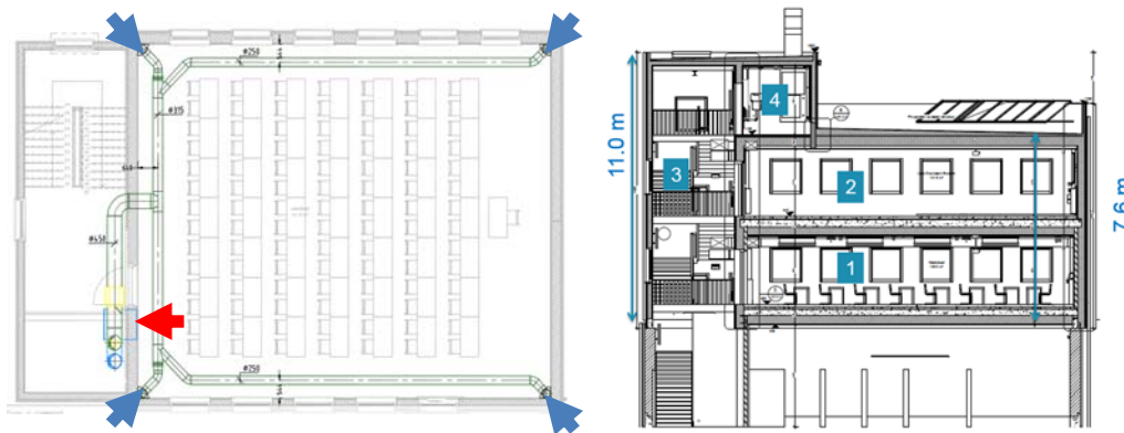
Figure 2; Left) Floor plan of the studied lecture room on the first floor, blue is supply air and red extraction air, Right) cross section of the building
