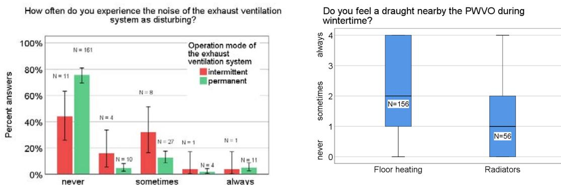
Figure 2: Left: Disturbing noise according to the operation mode of the exhaust ventilation system. Right: Assessment of draught according to the heat distribution. Indication of error bars on 95 %-level.
