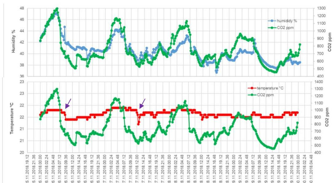
Figure 3: Measurement values from 25<sup>th</sup> through 30<sup>th</sup> November, 2018 from a bedroom in building type BB. Top: Humidity and CO<sub>2</sub>-concentration, bottom Temperature and CO<sub>2</sub>-concentration.
