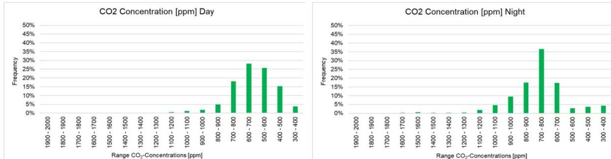
Figure 4: Left: CO<sub>2</sub>-concentrations during daytime (07:00-21:00) in a bedroom in building type BB (same flat as Figure 3) for the period of 19<sup>th</sup> of October 2018 to 29<sup>th</sup> of March 2019. CO<sub>2</sub>-concentrations during night time (22:00-06:00)
