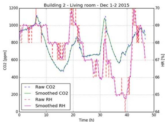
Figure 3: Example of smoothed time signal from raw data – CO<sub>2</sub> concentration on the left y-axis, RH (%) on the right y-axis. Measurement frequency of 5 minutes. Both signals have been smoothed using polynomial interpolation.
