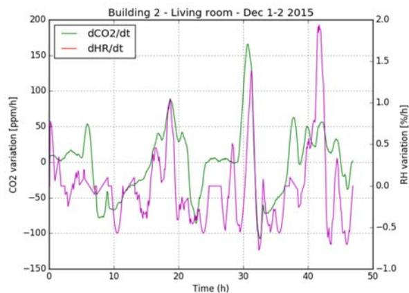
Figure 4: Time derivatives corresponding to Figure 3 smoothed signal.
