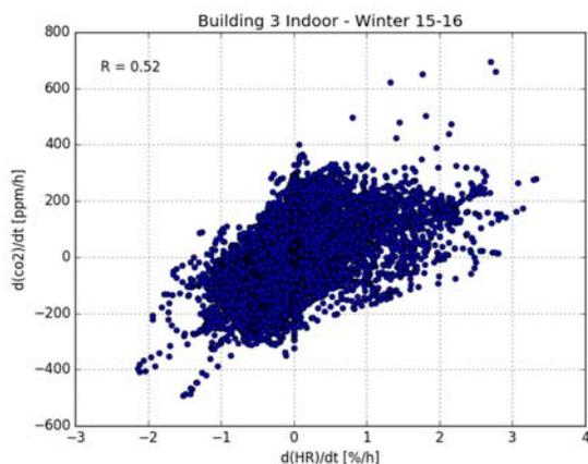
Figure 5: Correlation between CO<sub>2</sub> and RH time derivatives for one of the residential building on the 2015-2016 Winter months.
