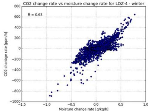
Figure 10: Room "LOZ-4" - CO<sub>2</sub> time derivative vs. moisture content time derivative for winter 2017-2018.
