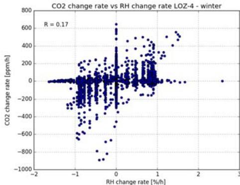
Figure 9: Room "LOZ-4" - CO<sub>2</sub> time derivative vs. RH time derivative for winter 2017-2018.
