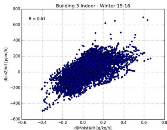
Figure 6: Correlation between CO<sub>2</sub> and Moisture content time derivatives for one of the residential building on the 2015-2016 Winter months.
