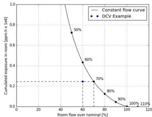
Figure 12: Comparison of DCV strategies with reference curve. In this example case, the DCV strategy (blue dot) gives IAQ equivalent to constant flow of 70% (of nominal), while the average flow over the period is only 60% of the nominal.
