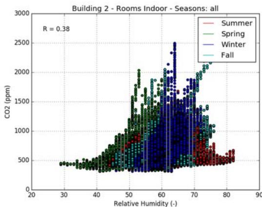
Figure 1: CO<sub>2</sub> vs. RH for living room of one of the residential buildings – A moderate linear trend is visible. While the maximum CO<sub>2</sub> levels are close for every season, the related RH are clearly different.
