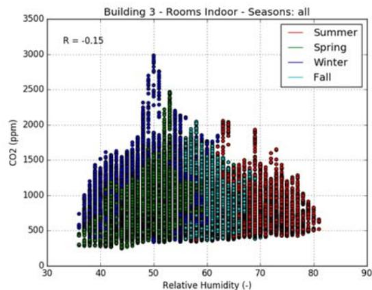
Figure 2: CO<sub>2</sub> vs. RH for living room of one of the residential buildings – The difference in RH values is clearly visible between the seasons, but there is not linear trend at all between the two variables.
