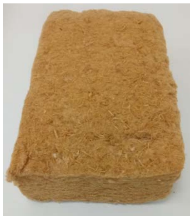
Figure1. Insulation bio-based board made of wood fibre
