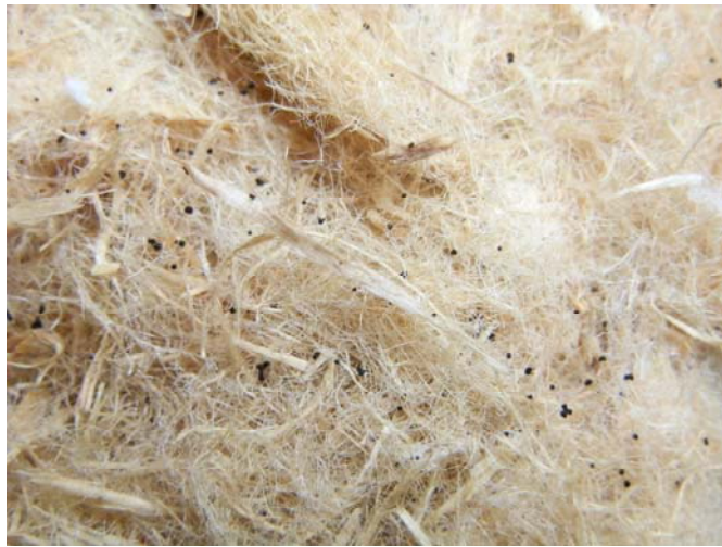
Figure 6. Colonies d' Aspergillus niger onto the material
