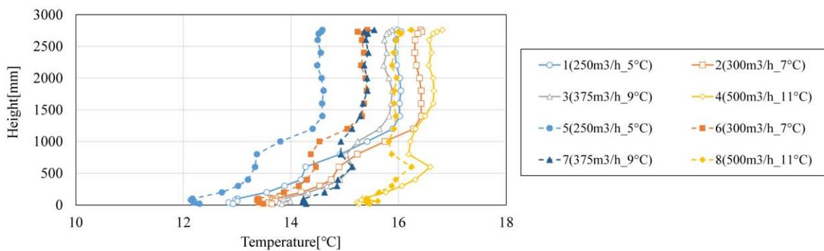
Figure 4: Vertical distribution of horizontal-averaged room Temperature
