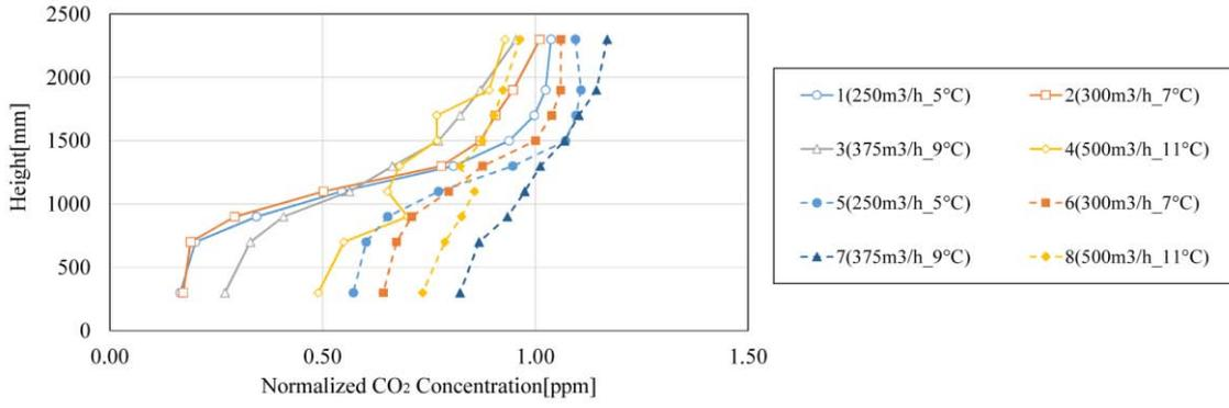
Figure 6: Vertical distribution of horizontal-averaged room Normalized CO<sub>2</sub> concentration
