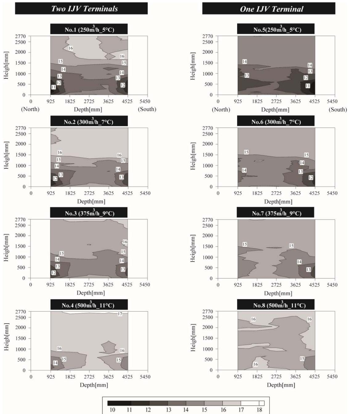
Figure 3: Temperature Contour
