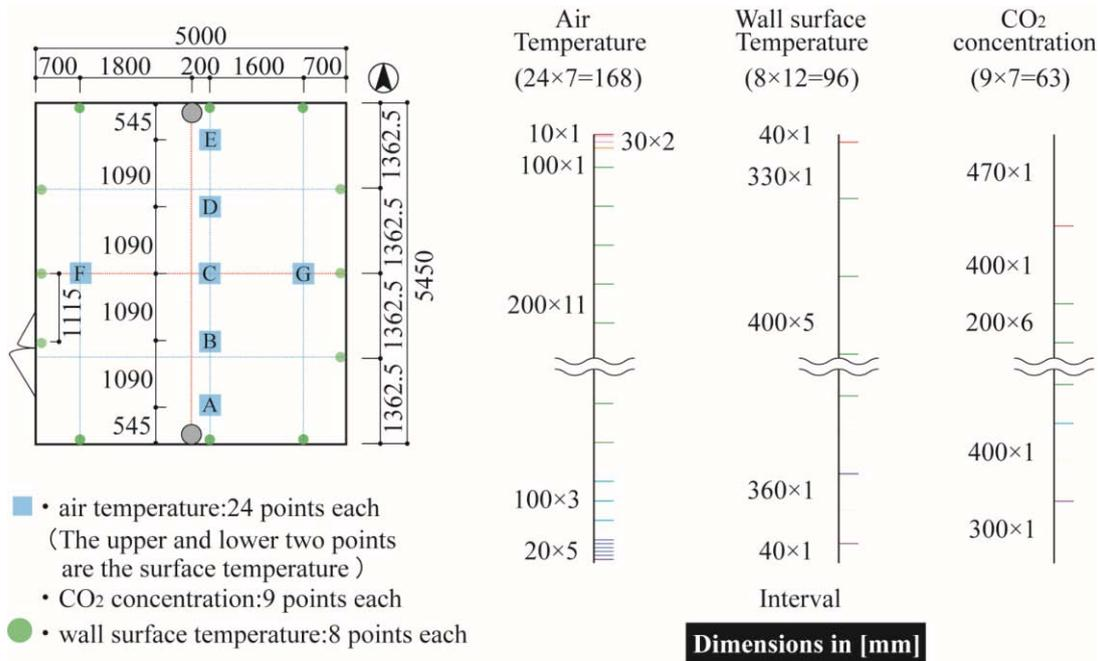
Figure 2: Measurement point of Temperature and CO<sub>2</sub> concentration
