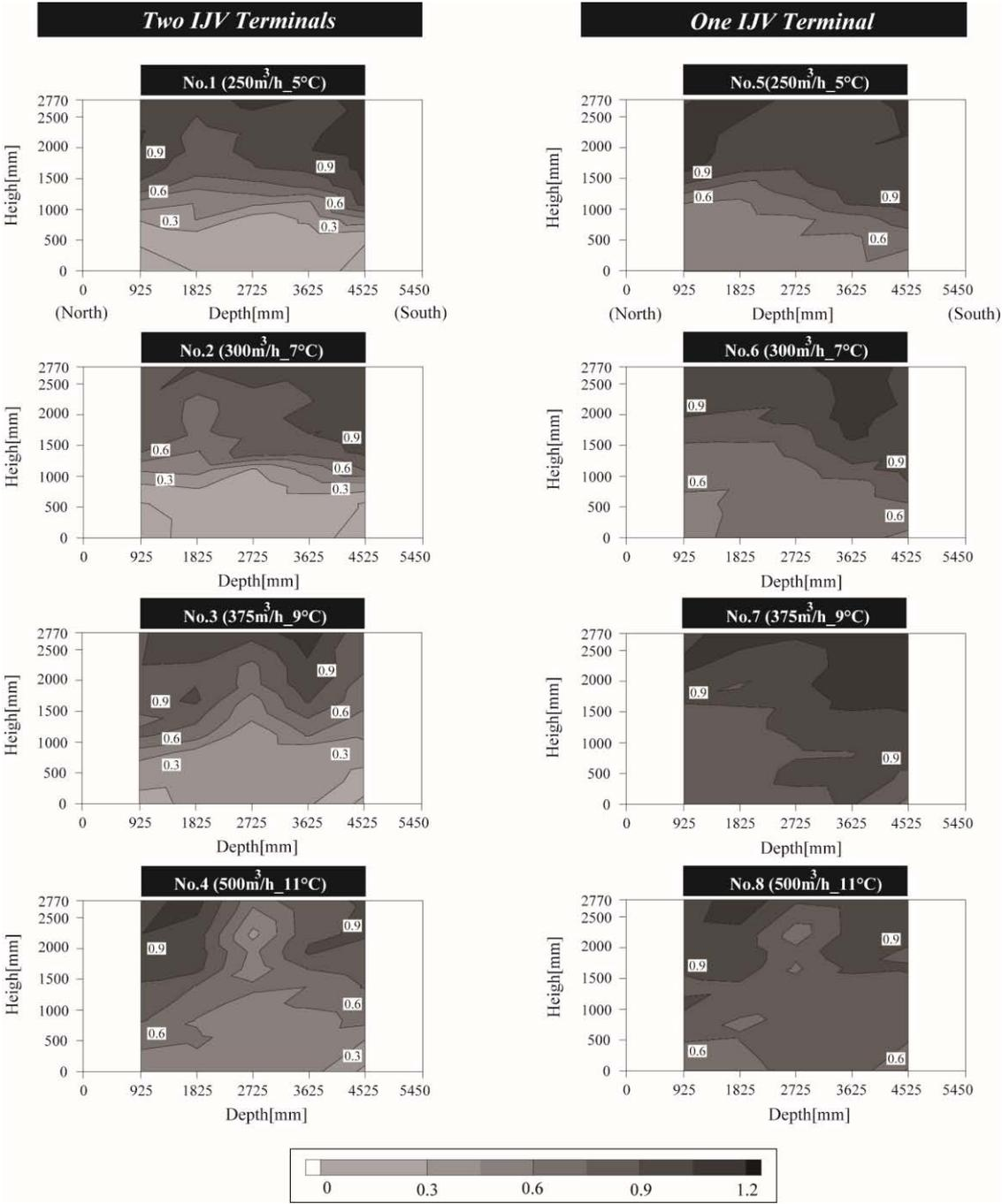
Figure 5: Normalized CO<sub>2</sub> concentration Contour
