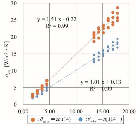
Figure 10 Correlation between Face Velocity and  $\alpha_{cm}$
