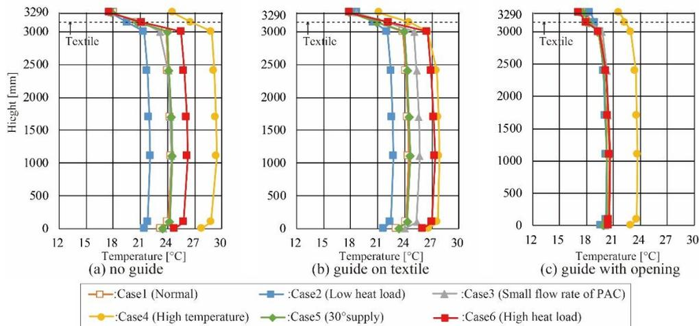
Figure 5: Vertical Temperature Distribution
