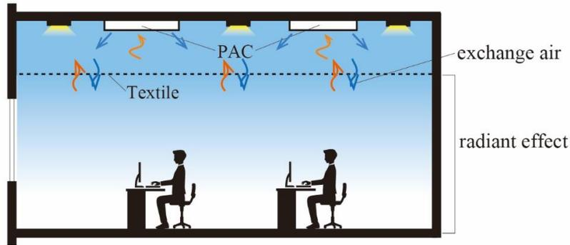
Figure 1: Outline of Ceiling Radiant Textile Air Conditioning System with PAC
