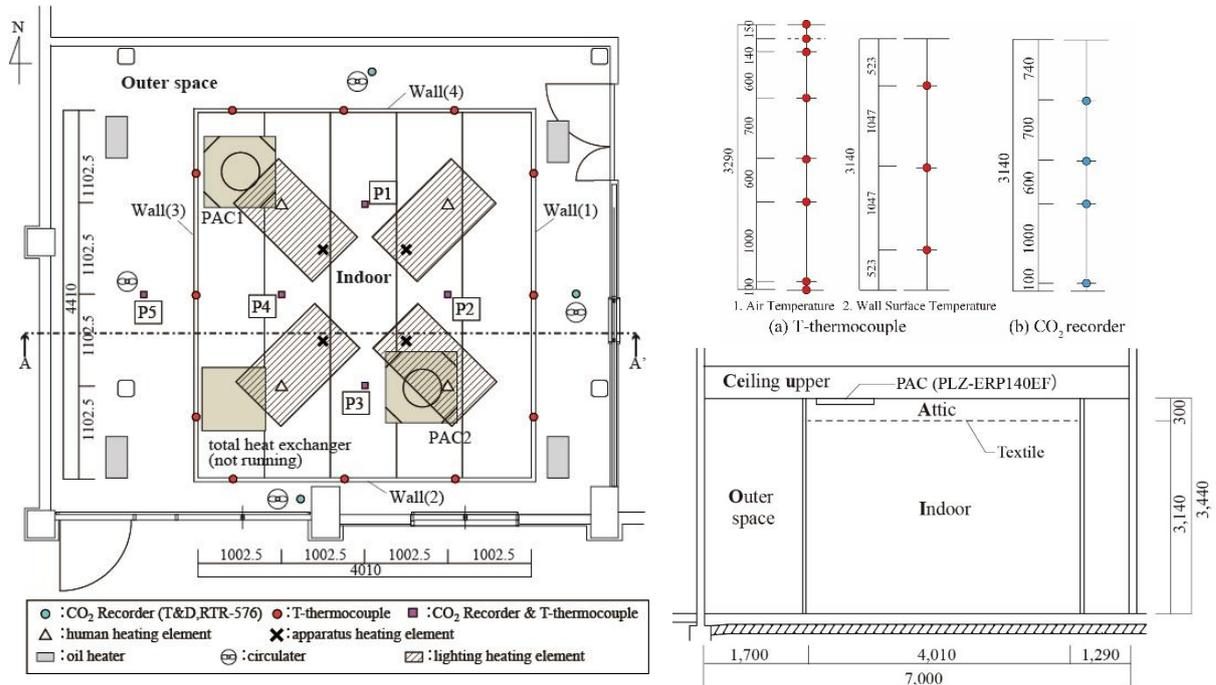
Figure 2: Plan of Experiment Room and A-A' Elevation and Measurement Points
