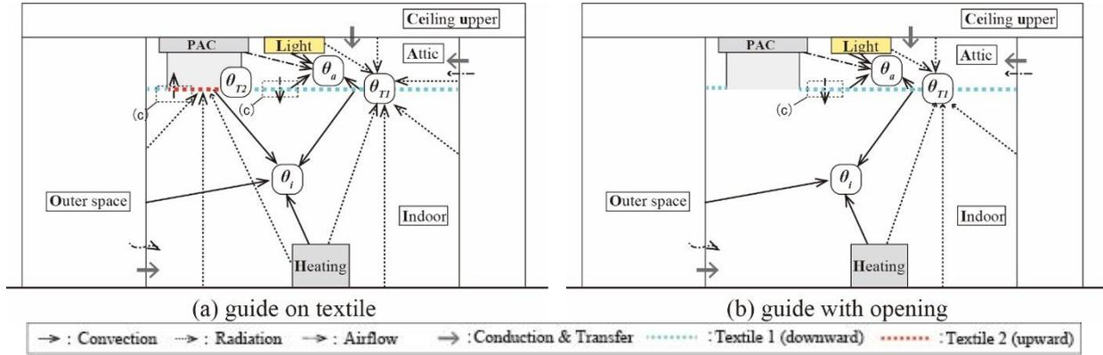
Figure 7: Modelling of Heat Transfer of this System
