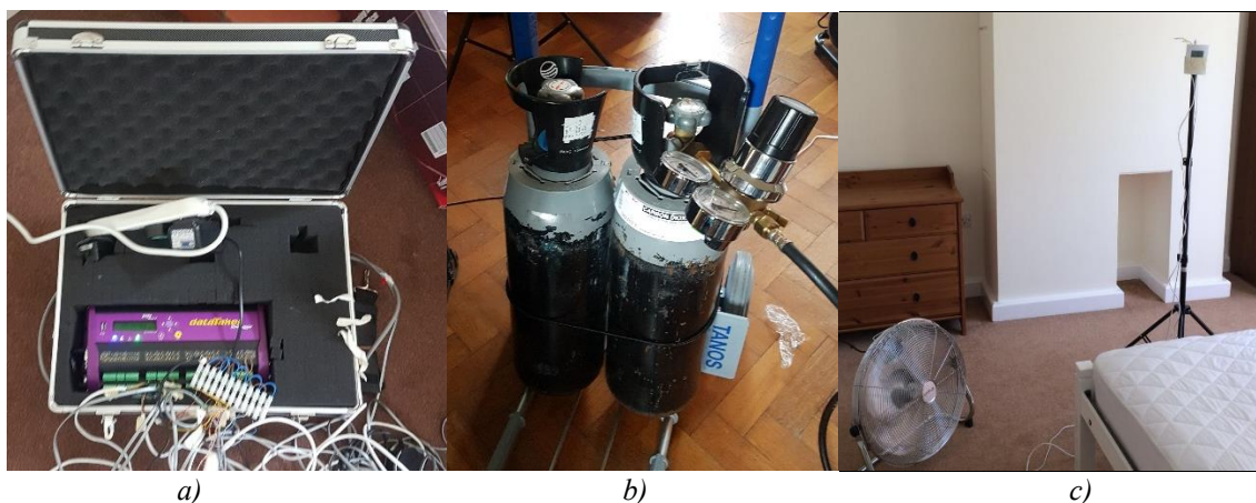
Figure 1. Equipment utilised for tracer gas decay method tests. a) Data logger with sensors connections, b) carbon dioxide canisters, c) example of a building zone, with a temperature sensor, a carbon dioxide sensor and a fan.
