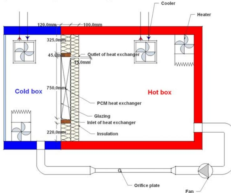
Figure 3: Experimental setup for the test of PCM heat exchanger prototype. Figure comes from (Hu and Heiselberg, 2018)
