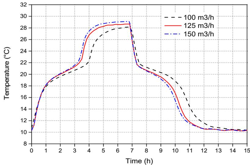
Figure 7: PCM temperature with different flow rates
