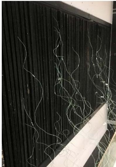
Figure 4: Setup of thermal couples in the heat exchanger
