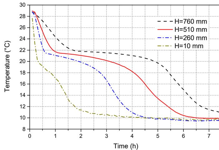
Figure 5: The temperature distributions along the height of one plate in the freezing process
