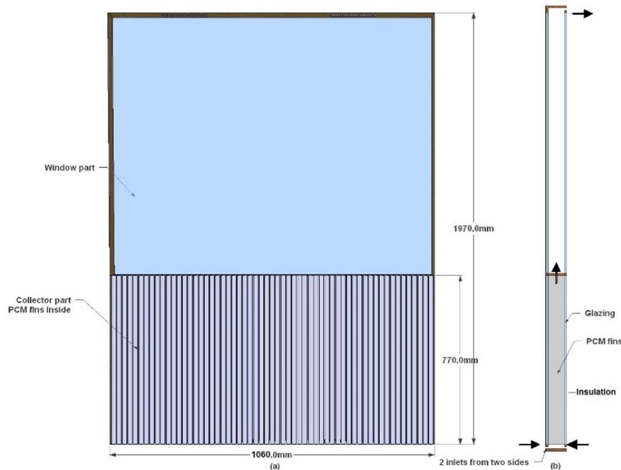
Figure 1: The sketch of the ventilated window with a PCM heat exchanger. Figure comes from (Hu and Heiselberg, 2018)
