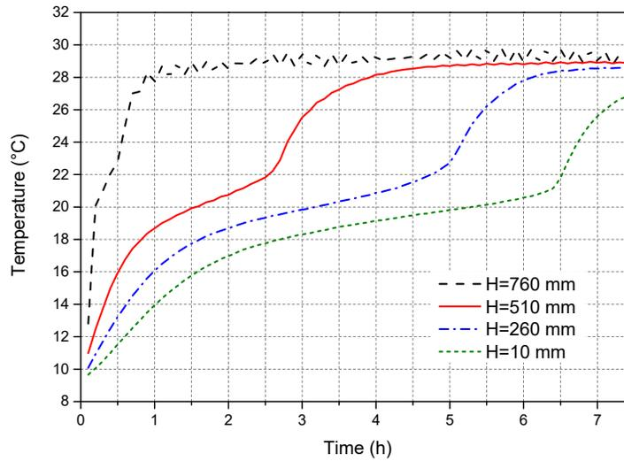
Figure 6: The temperature distributions along the height of one plate in the melting process
