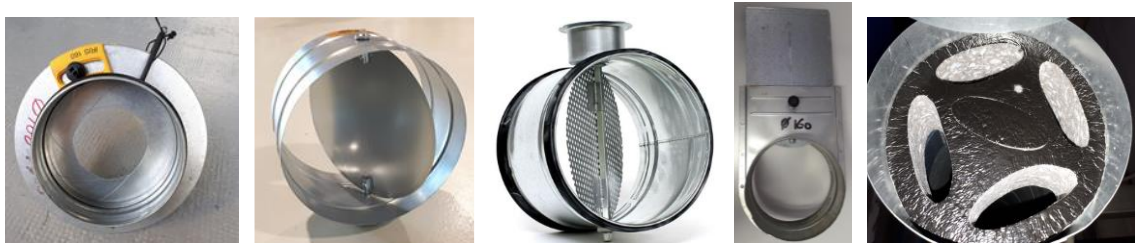
Figure 10: tested dampers (l. to r.): iris damper, damper blade (full or perforated), blast gate, flexible opening foam
