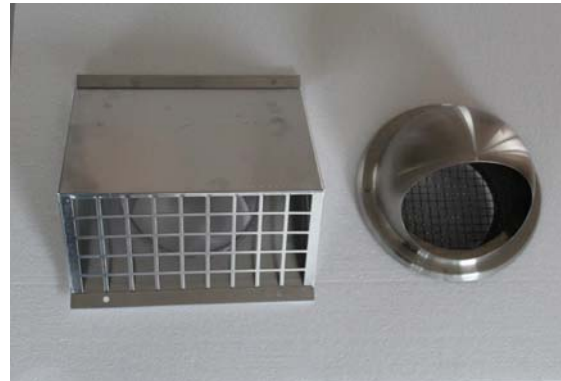
Figure 2: Comparison of the externally mounted air transfer devices before (right) and after (left) optimisation in step 2.
