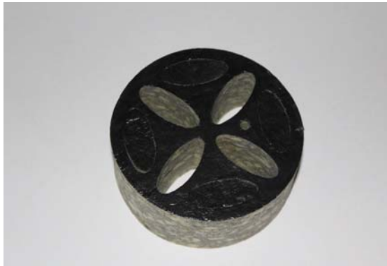
Figure 1: Foam sound attenuator initially used behind the ATD of the living room.
