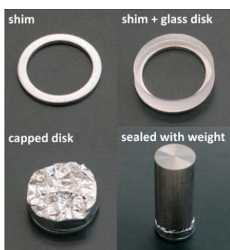
Figure 4: Elements of the diffusion chamber sampler for measuring K_s .
