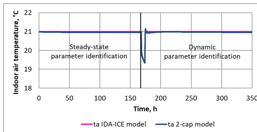
Figure 4: Steady-state and dynamic parameter identification in RC-model calibration with constant  $T_{out} = 18 \text{ }^\circ\text{C}$ .
