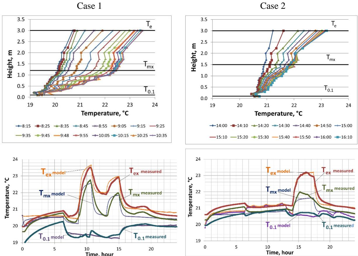
Figure 5: The measured indoor temperature profiles (upper) and the comparison of the two-capacity model three temperatures with measurements (lower).
